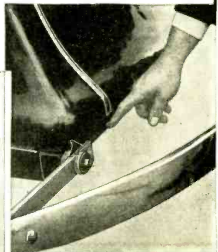
Finger points to insulated bushing supporting the rear bumper; this insulated bumper acts as the "antenna." The wire connecting the insulated bumper to the transmitter can be clearly seen and also the insulating washers.
