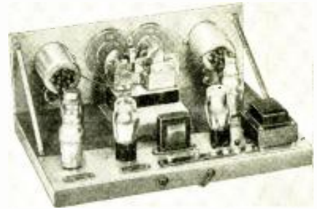
Right-front and rear views of 5-tube Mascot receiver; has a stage of tuned R.F. detector and two stages of audio, completely A.C. operated. Dynamic or magnetic speaker can be used.
