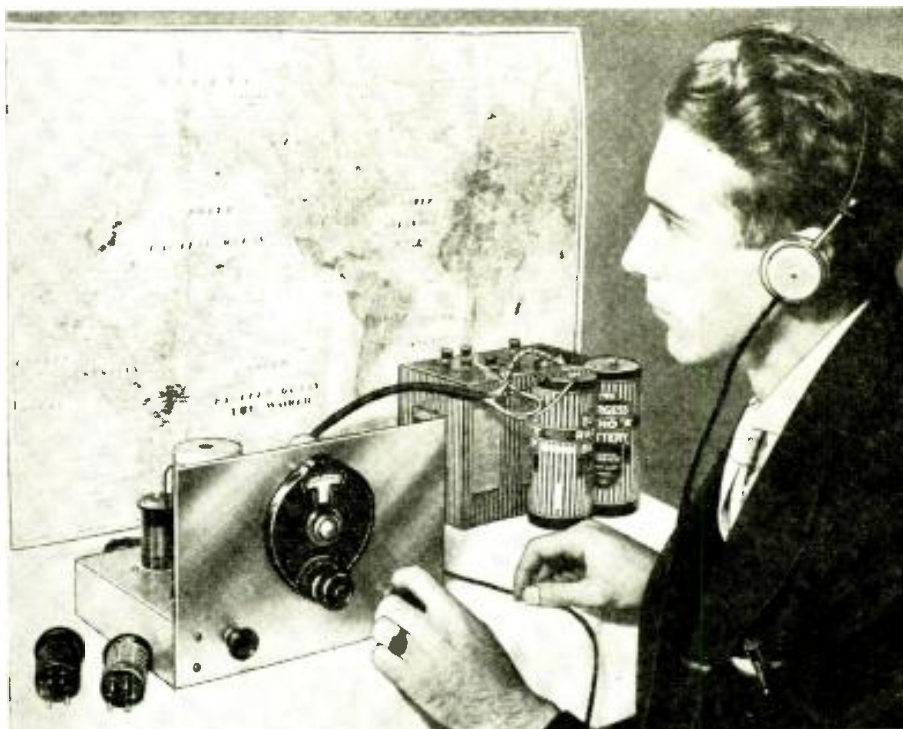
The designer of the "3-tube equals 5" Battery Receiver, which features the use of a separate regeneration triode, is here shown giving the set its final test. "O.K." says W2AMN.
