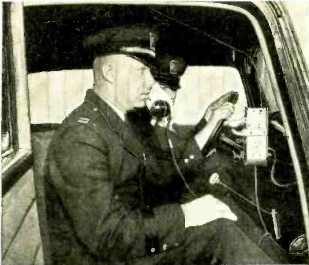
Captain Walter Kirchoff of the New Rochelle, N. Y., Police Department, using the new French type radio telephone; note hook on dash.
